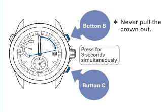
\* During movement of the date, the buttons cannot be operated.
