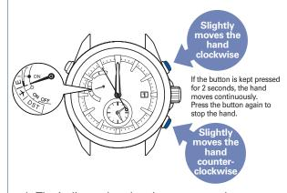
\* The indicator hand makes one complete turn, but this does not mean a failure.
