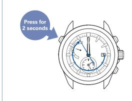
\* If no operation is performed for more than 1 minute or when Button A is pressed once, the watch returns to the time display mode.
